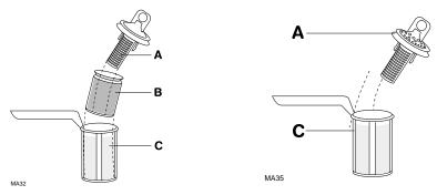
3. Turn the handle about 1/4 a turn anticlockwise and remove.
